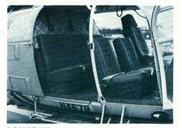
COMFORT: "Room to spare" describes the seating in the Alouette 3. With no center frame supports to get in the way, you can enjoy an unrestricted view. Soundproofing allows for ease of conversation throughout its spacious cabin. Wide sliding doors and a sturdy passenger step make entry and exit the easiest ever.
